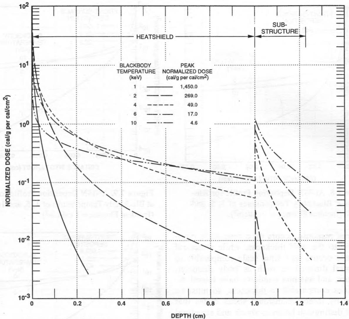
**Figure 7.11.** X-Ray Energy Deposition in a Typical Heatshield and Substructure for Blackbody Temperatures From Cold to Hot (1 to 10 keV) (Doses Normalized to an Incident Fluence of 1 cal/cm<sup>2</sup>).
